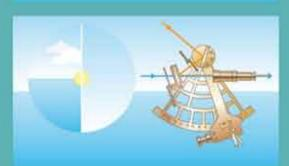
2. As the index bar is moved, the image through the viewfinder splits in two and the Sun is brought down to the horizon. The angle can be read off the curved scale and converted into the altitude of the Sun above the horizon.
